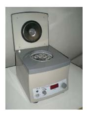
The Serrata Laboratory centrifuge operates on 230-240VAC and uses 12 x 20ml standard centrifuge tubes inclined into the top rotor.
